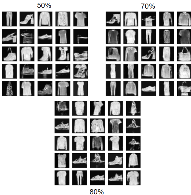
Fig. 5. Outputs from the channel-pruned DCGAN model trained on Fashion-MNIST
